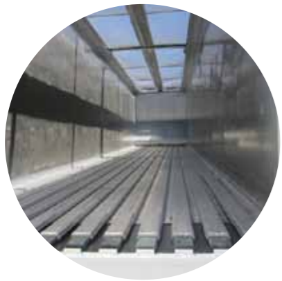
Fully Sealed Sub Deck
